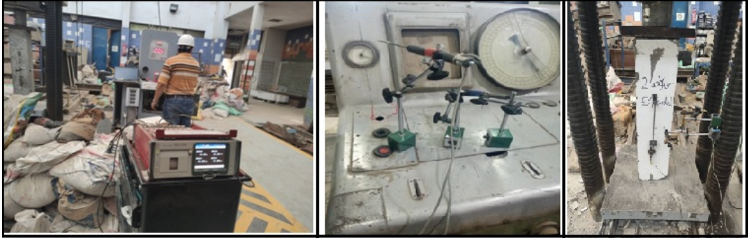
Fig. 5. Testing Machine, Data logger device and the positions of axial and lateral LVDTs on tested column
