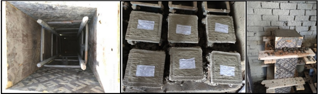
Fig. 3. Preparing of steel cage, casting, and curing of the tested columns.
